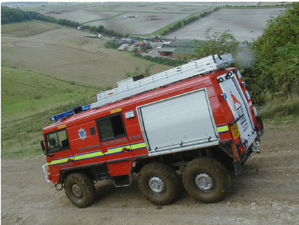
The Pinzgauer six wheel-drive off-road pumping appliance
